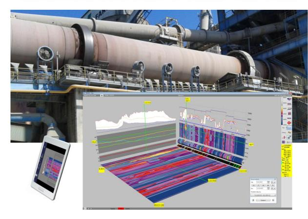
New system can be integrated into modern networks and mobile configurations using newly applied transparent 3D graphics and enhanced diagnostics of kiln status
